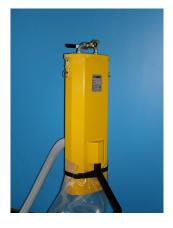
The compact design makes the MACRO light weight and easy to move and carry. During use the MACRO is positioned on a sturdy stand which allows easy access for changing the plastic bag which collects the rock cuttings and dust.
