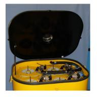
Easy access to filters and air valves by opening the top, the clean side of the dust collector.
